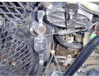
This is the bottom of the regulator. You can see how the line goes into the filter, then the solenoid, then the reg. The solenoid gets wired to a key on 12v. It is very low amps.
