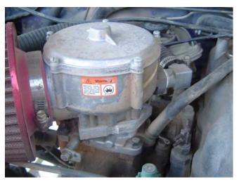
This is the mixer assembly bolted on the factory carb base. You'll notice we reused the factory carb base for its unique throttle and pcv mounting. You will need to reuse the three factory screws that bolt the base to the adapter.
