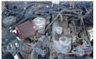
These are the hoses connected and the kit installed. Notice the vacuum advance is connected to the forward port on the distributor. This port is the advance. The other end connects to a ported vacuum source on the carb base.
